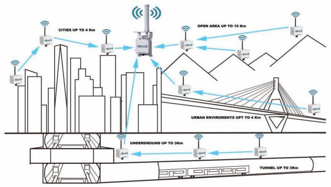
The DMS Mesh network allows all our Nodes to talk to each other, thus allowing them to relay other Nodes' data to the gateway. Challenging sites like deep tunnels and large mines can be monitored easily with a multi-hop wireless mesh network.
